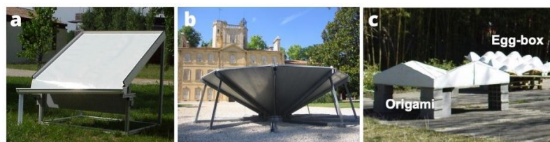
Figure 3. Various dew collectors: a: Plan; b: Cone [Source: Photo O.Clus]; c: Origami and egg-box [Source: Photo D.Beysens]
