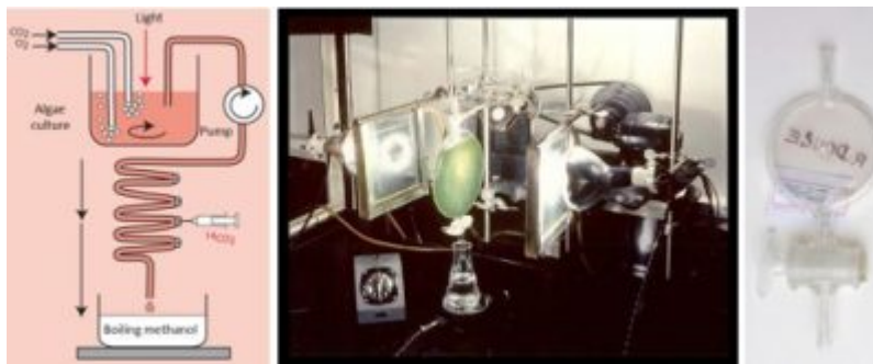
Figure 2. Diagram of the apparatus used to monitor the incorporation of photosynthetic carbon into the products of photosynthesis . In the centre: device used for the study of CO 2 fixation by unicellular algae. [Source Photo © Ernest O. Lawrence, Berkeley National Laboratory, Photography and Digital Imaging Services: previously unpublished, Biochemistry & Molecular Biology of Plants . B.B. Buchanan, W. Gruissem & R.L. Jones. American Society of Plant Physiologists, Rockville, MD. 2000 p. 610]. Right: Lollipop given to Pr. Roland Douce by Andrew A. Benson and kept at the Musée des Confluences (Lyon, France).
