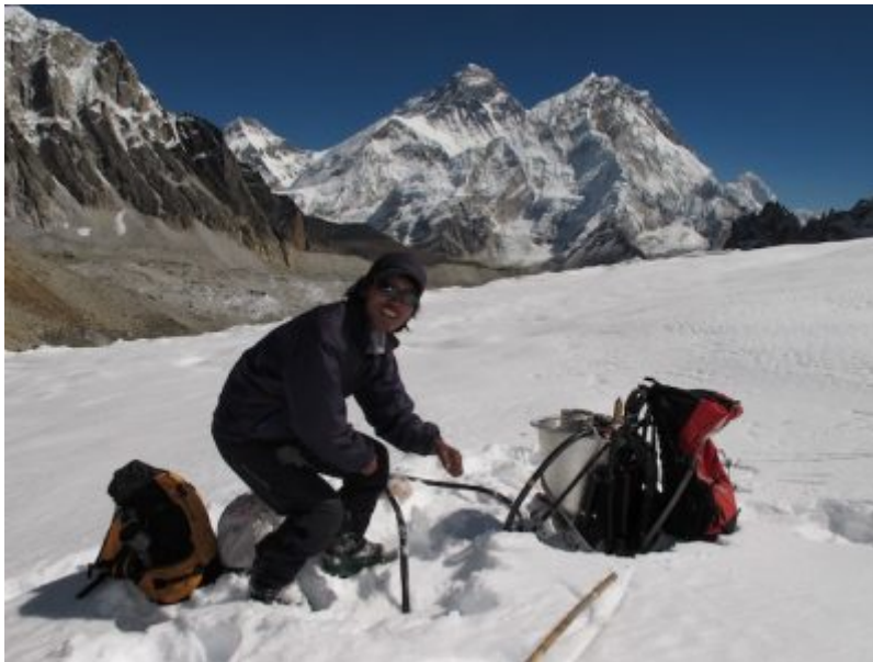
Figure 1: Installation of a bamboo ablation stake with a steam drill in the ablation zone of the West Changri Nup Glacier, with Mount Everest visible in the background. [Source: © Patrick Wagnon]
