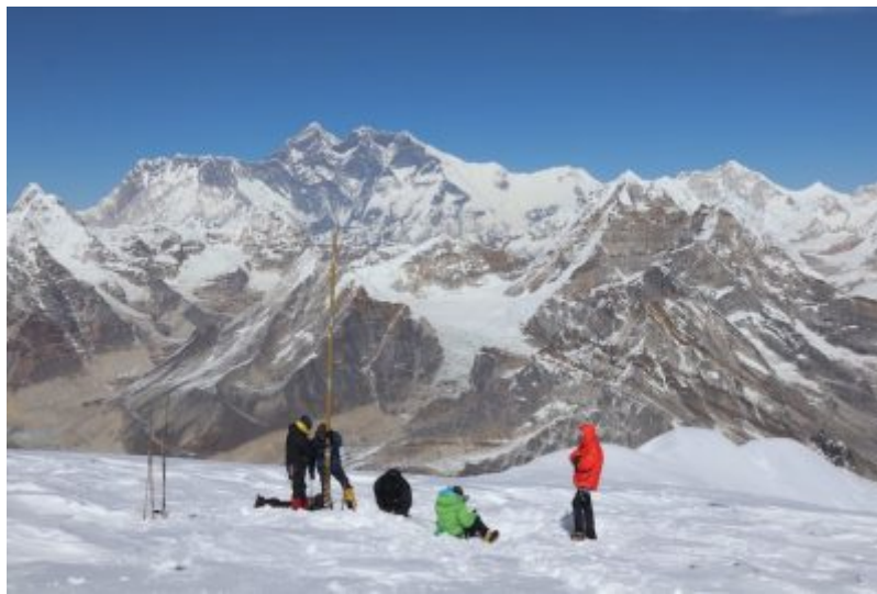
Figure 2: Measurement of point mass balance using a corer coupled with density measurements in the accumulation zone of the Mera glacier at 6350 m altitude, a.s.l., with Mount Everest visible in the background. [Source: © Bruno Jourdain]
