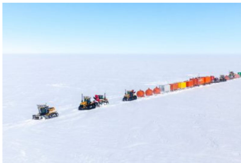
Figure 4. Land convoy linking Robert Guillard station, an annex of Dumont d'Urville station in Terre Adélie, to Cap Prudhomme, and Concordia station, 1100 km apart. All of Concordia's supplies, fuel, food, building materials, scientific equipment, are provided in this way, through 2 to 3 trips during each austral summer. The staff are transported by plane. [Source: © Thibaut Vergoz - IPEV]
