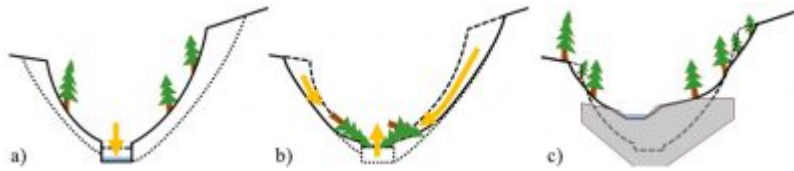
Figure 1. Bed stabilization: Diagram of a profile across torrents showing the effect of longitudinal profile erosions and the origin of certain respirations of the bed: a) erosion of the bed leading to a lowering of its level, this erosion leads to b) lateral instabilities; these two processes being stabilized by c) the installation of an adapted dam: built above the original bed, preventing bank erosion and destabilization and moving the bed axis to the bank least susceptible to erosion. [Source: © G. Piton]
