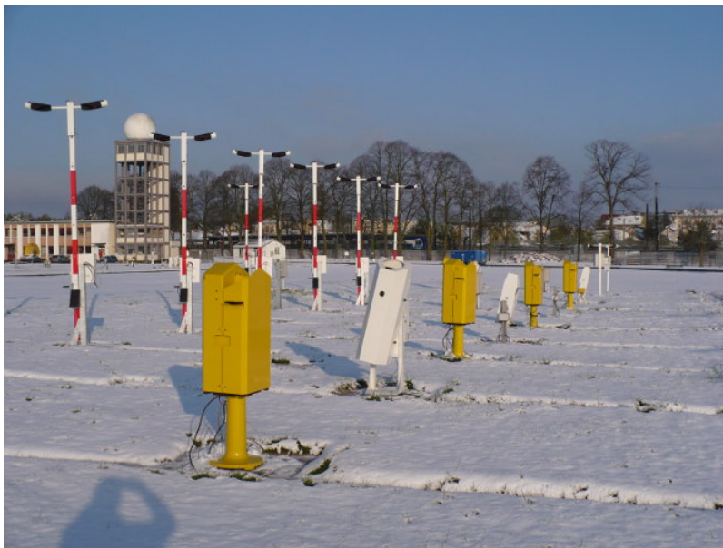
Figure 12. Cloud rangefinders. [Source : © Michel Leroy]
