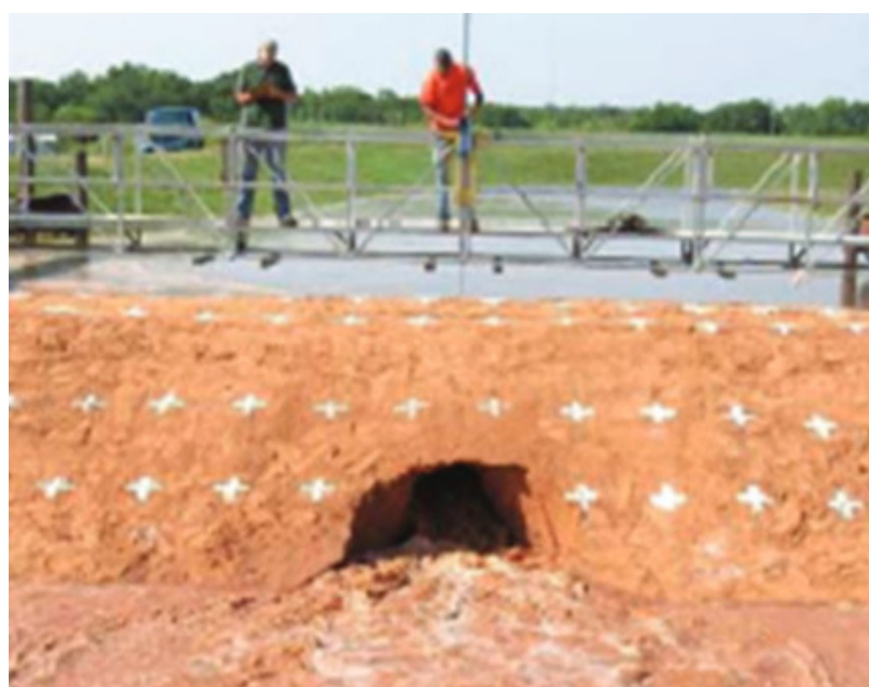
Figure 3: Example of a piping erosion test [photo from Hanson et al. (2010)[6], USDA Agricultural Research Service credit].
