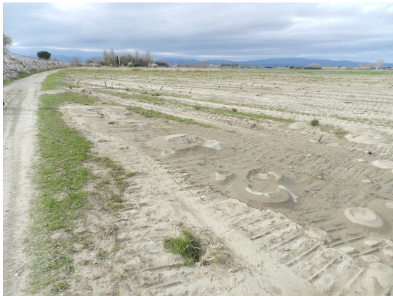
Figure 2: Example of a sand mound resulting from a "sand boil" downstream of a dyke (Agly dyke, March 2013) [Source: © P. Mériaux].
