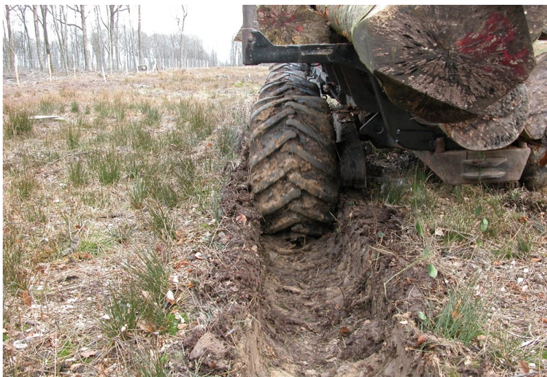
Figure 10. Ruting caused by timber unloading in a forest environment. Deep horizons can be affected by irreversible compaction. [Source: © Jacques Ranger, with the author's permission]
