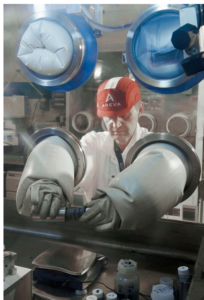
Figure 10. Glove boxes for handling radioactive products, Mox fuel fabrication plant [Source: 102723 © LARRAYADIEU Eric / AREVA]
