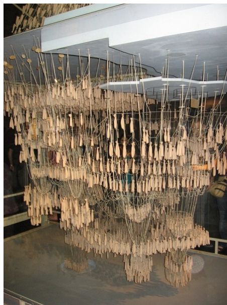
Figure 2. Inverted model of Gaudi's Sagrada Familia Cathedral. The equilibrium shape is such that at each wire intersection the vector sum of the forces is equal to zero. Each beam element is represented by a wire, and its mass simulated by a weight. The tension force on a yarn is necessarily aligned with the yarn. In the actual inverted configuration, the corresponding force will then be a compression force aligned along the beam, which guarantees its mechanical strength. [Source: http://olive-art.weebly.com/uploads/2/16/10/5/26053332/6555663_orig.jpg ].
