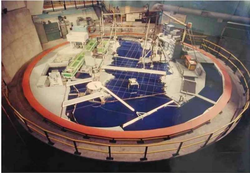
Figure 4. Physical scale model of the English Channel on the large "Coriolis" rotating platform at Grenoble, France.
